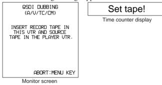
7 Insert the source tape in the player, and the recording tape in this unit.
